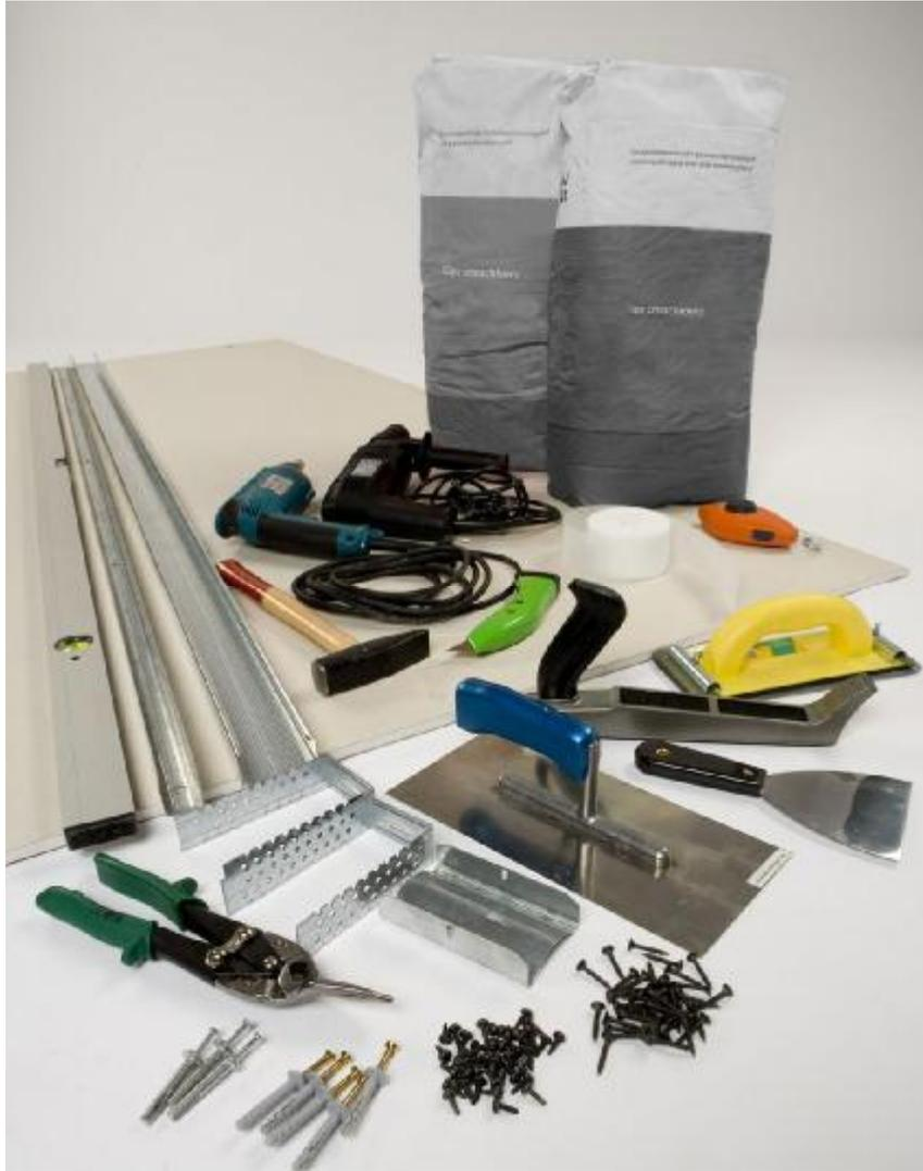
Fig. 8. Tools and materials used in interior drywall systems
